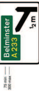
2101.1 Grade separated junction ahead of a non-primary route and a primary route
